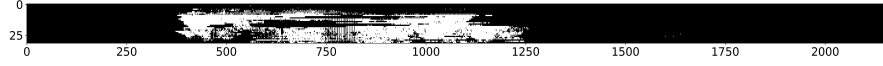
Fig. 5: Mask of LiDAR image (class for each of the pixels). White: particle , black: non-particle .
