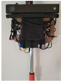
Fig. 2: A Kinect One (v2) sensor mounted on a garden pole used for hand-held scanning of trees. The device is powered using a portable battery.
