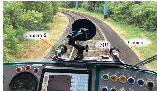
Fig. 1. Datasets recorded with a custom sensor setup for visual-aided odometry in sub-urban and industrial environments are used for evaluation of popular visual-aided odometry frameworks for rail applications. We show that high accuracy motion estimation can be achieved using stereo vision. Furthermore, incorporating inertial measurements increases accuracy and robustness.
