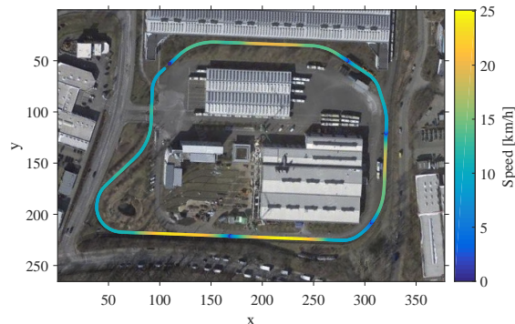
Fig. 3. Trajectory1 around the depot in an industrial environment with speeds up to 25.5 km/h.
