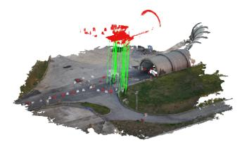
Fig. 1: Global localization of a 3D UGV sub-map (red point-cloud) in a 3D UAV reference map (coloured point-cloud). Green lines indicate the resulting matches associated to points in the two point-clouds. The data stems from the Montelibretti outdoor dataset and drawn from the complex experimental set-up.
