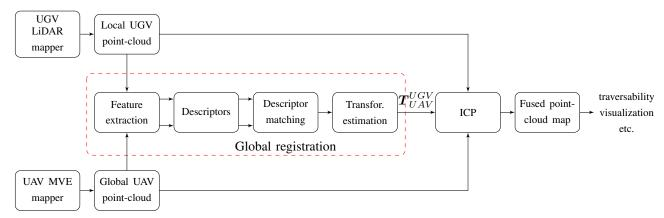
Fig. 2: Mapping System overview. The inputs to the system are the local UGV map and the global UAV reference map. If a global registration is triggered, the key-points are computed on both maps. Consecutively, the system performs descriptor extraction and matching. The initial global transformation is then refined by a step of ICP between the global and the local clouds, resulting in a fused map that is used for further functionalities of the system, such as path planning.
