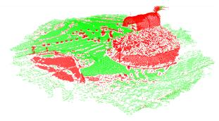
Fig. 3: Resulting UGV traversability estimation on the outdoor Montelibretti dataset. Traversable areas are marked in green, while non traversable areas are indicated with red. The parametrization is identical to the parametrization for LiDAR traversability analysis.
