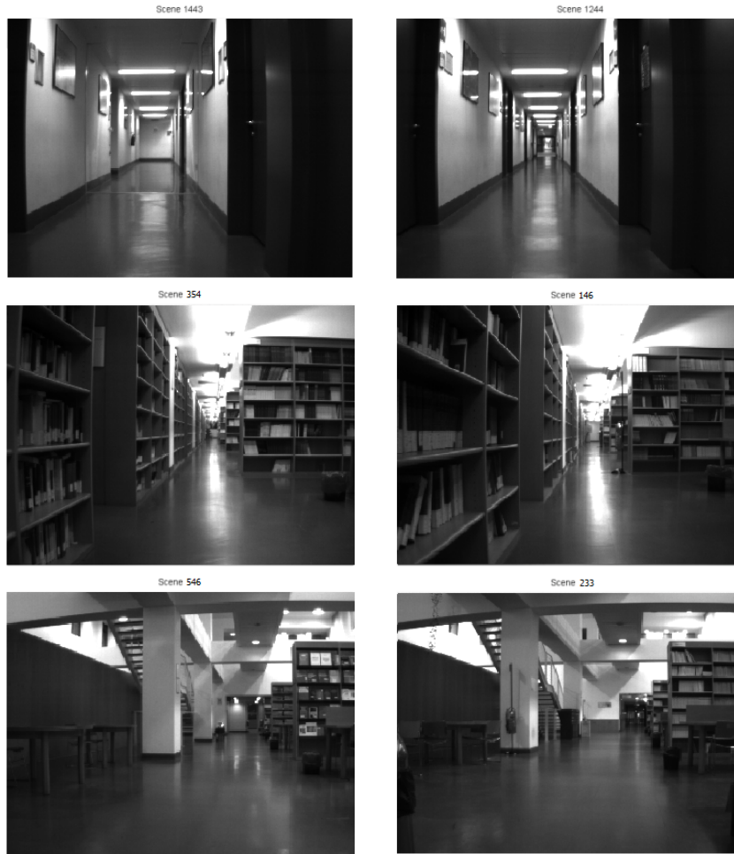
Figure 3.13: Three of the false positive cases that the FAB-MAP and BoW plus epipolar constraint obtain in the indoor dataset.
