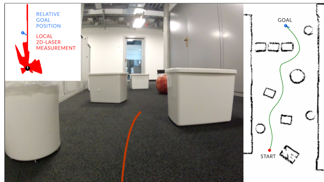
Fig. 1: The robotic platform is able to safely navigate through a maze-like environment only using local laser and target information (upper left). The final traversed trajectory is visualized on the map (right). The robot view image is only shown for visualization purposes but not used as an input to the end-to-end algorithm.
