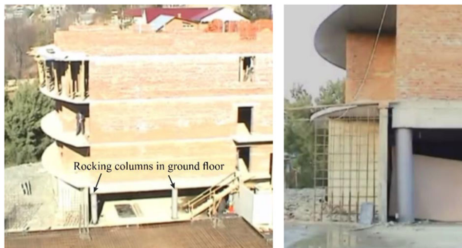
Figure 1. Full-scale dynamic tests of a rocking podium structure [14]: four-story masonry structure (left) and initial displacement of the ‘kinematic bearing’ story column (right).
