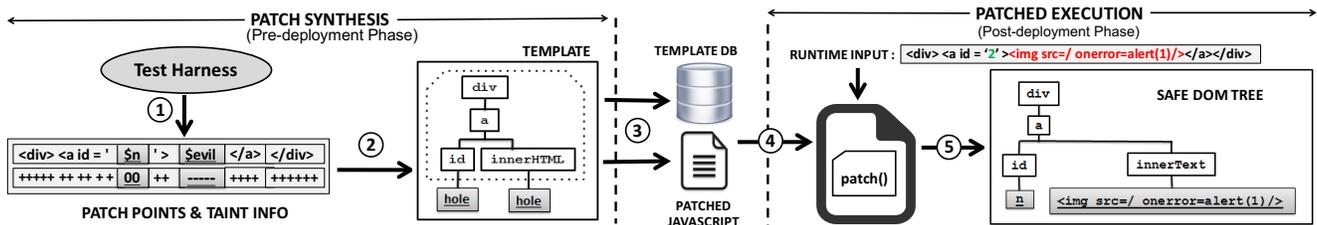
Figure 3: Approach overview of DEXTERJS: (1) Patch point identification (2) Template Inference (3) Hot-patching (4) Template selection (5) Runtime template instantiation for safe DOM rendering.
