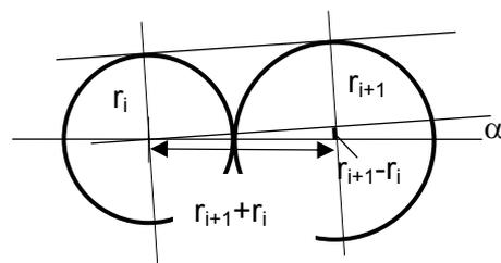
$$\sin \alpha = \frac{r_{i+1} - r_i}{r_{i+1} + r_i} = \frac{\sqrt{k_H} - 1}{\sqrt{k_H} + 1} = \frac{0.18}{2.18} = 0.0826 \rightarrow \alpha = 4.74^\circ$$
