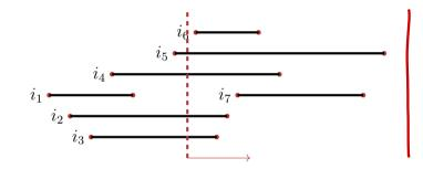
Idea of a sweep line: vertical line, moving in *x*-direction, observes the geometric objects.
