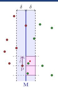
Which points are relevant for point p?  $\Rightarrow$  the ones in a circle around p with radius  $\delta$  **Observation 1:** The relevant points are contained in two ( $\delta \times \delta$ )-rectangles.
