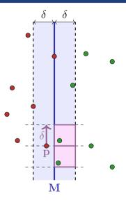
Which points are relevant for point p?  $\Rightarrow$  the ones in a circle around p with radius  $\delta$  **Observation 1:** The relevant points are contained in two ( $\delta \times \delta$ )-rectangles.
