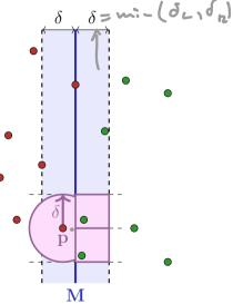
Which points are relevant for point p?  $\Rightarrow$  the ones in a circle around p with radius  $\delta$  **Observation 1:** The relevant points are contained in two ( $\delta \times \delta$ )-rectangles.
