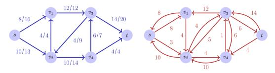
Residual networks provide the same kind of properties as flow networks with the exception of permitting antiparallel edges
