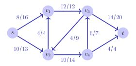
Residual networks provide the same kind of properties as flow networks with the exception of permitting antiparallel edges
