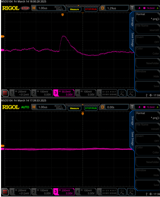
Fig. 2 | Shaper configuration used to measure the particle hits of the ^{90}\text{Sr} source:
