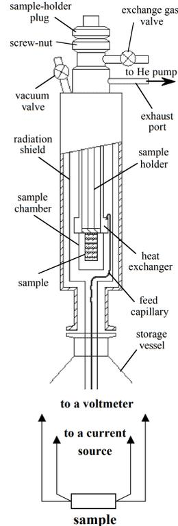
**Fig. 1** | Sketch of the continuous flow cryostat used in the experiment after inserting the feed capillary in the storage vessel to allow for temperature exchange with the sample located in the sample chamber. Additionally the wiring for a 4-point measurement is sketched below the continuous flow
