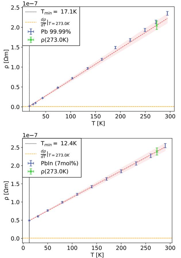
**Fig. 2** | Measured resistivity of the samples Pb and PbIn (7mol%) as a function of temperature down to  $T_{min}$ . The linear fit is shown in red with the error of the fit indicated by the shaded area. Additionally marked in green is the value for the resistivity at 273.0K which was not measured but calculated using the linear fit performed on the measured dataset for each sample.
