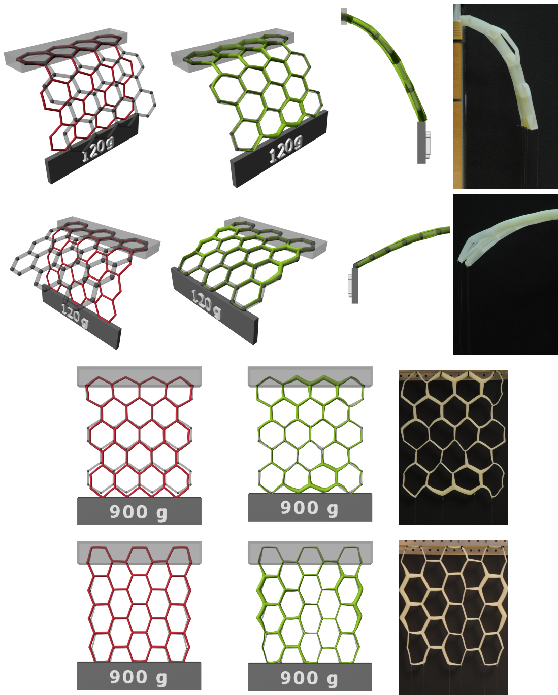
Figure 6: Resulting deformations for each of the four target poses of the sheet demo. Default deformations (in red) are compared against the optimized results obtained using our framework (in green). Last column shows the physical printed sheet matching the behavior predicted by the simulation model. Target configurations of the rod mesh are shown in light transparent gray.
