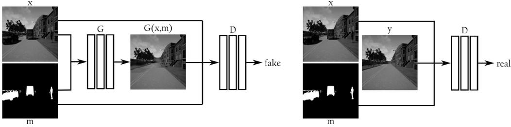
Fig. 4: The discriminator  $D$  has to learn to differ between the real images ( $y$ ) and the images produced by the generator ( $G(x; m)$ ).  $D$  is conditioned by both the dynamic/static binary mask  $m$  and the input image  $x$  to make a better decision about the origin of the image.
