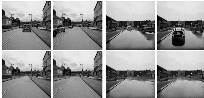
Fig. 1: Images at the same location with different dynamic content such as cars or pedestrians (top row) can be converted into the same static image, *i.e.*, a dynamic-object-invariant space (bottom row).
