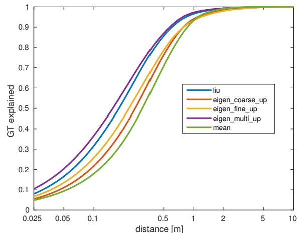
**Fig. 8:** Performance of full resolution depth estimates: liu [10], eigen\_coarse and eigen\_fine [4], eigen\_multi [3]
