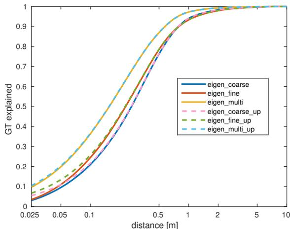
**Fig. 7:** Performance of original and full resolution depth estimates: eigen\_coarse and eigen\_fine [4], eigen\_multi [3], **\_up** indicates upscaling to the ground truth resolution
