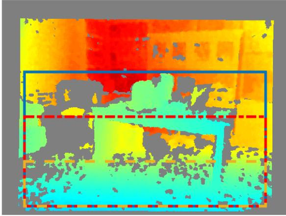
**Fig. 2:** We evaluate the effect of three different partial coverages of the scene. In the figure we show one depth image with rectangles covering the 53% (blue, solid line), 35% (red, dot-dashed line) and 18% (yellow, dashed line) of the full scene.
