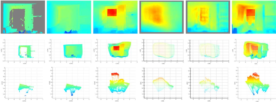
**Fig. 6:** One example from the NYU-V2 test set. *Left to Right:* Ground truth, Inpainted Ground Truth, Liu *et al.* [10], Eigen *et al.* [4] coarse, Eigen *et al.* [4] fine, and Eigen and Fergus [3]. *From top to bottom :* Depth Image, XY-view and XZ-view of the point cloud. The corresponding RGB image is shown in Fig. 1.
