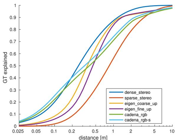
Fig. 11: Performance of full resolution for two stereo densities (dense and sparse), eigen\_coarse and eigen\_fine [4].
