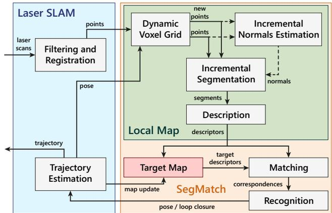
Fig. 2: Architecture of the incremental segment matching pipeline and its interface with a laser SLAM framework<sup>1</sup>.
