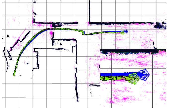
Figure 5: Comparison of drift in single session visual SLAM against 2D LiDAR scan matcher over a 20m trajectory. Grid scale is 2m. (For interpretation of the references to colour in the text, the reader is referred to the web version of this article.)
