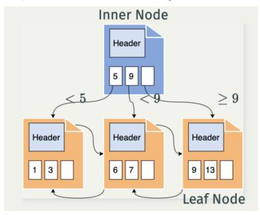
This tree structure allows us to perform search, insertion and deletion in  $\mathcal{O}(\log_M N)$ , where M is the maximum number of children per node.
