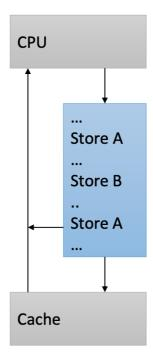
We want to avoid stalling the CPU for memory writes. We introduce a FIFO queue to buffer writes. When we want to read a address that has a yet completed write, we can directly read out of the write buffer.
