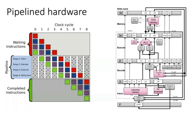
Pipelined processors are already a lot fast, but they introduce data / control hazards that need to be dealt with.
