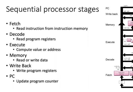
Such a sequential processor is slow, this is due to the fact that a signal has to propagate through every stage in one cycle. The clock therefore can't go very fast and single hardware units are only active for a fraction of the cycle.
