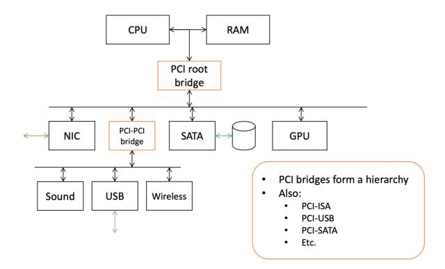
Each PCI device asks for a set of address ranges. The bridges up the tree remap addresses to the device. As a result each device appears as a set of contiguous address ranges.
