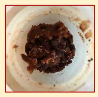
1. We synthesised Fh in the laboratory. Porous PETE sachets (dimensions approximately  $30 \text{ mm} \times 12$ mm  $\times$  3 mm, pore size 52  $\mu$ m) were filled with ~0.5g of Fh.
