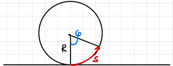
$$\begin{aligned} \text{Eigendrehmoment} &= M = J \cdot \ddot{\varphi} \\ \text{"- Drehimpuls} &= L = J \cdot \dot{\varphi} \end{aligned}$$
