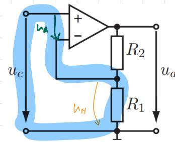
$$\text{NICHT INVERTIEREND: } u_a = \frac{R_1}{R_1 + R_2} u_e \quad u_a = u_e - u_N = u_e - u_a \frac{R_1}{R_1 + R_2}$$
