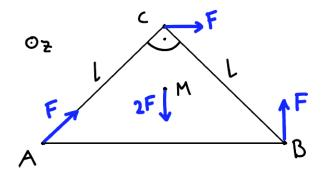
Berechne das Moment in A, B & C. Lösung:  $M_A = -\frac{\sqrt{2}}{2}lF$ ,  $M_B = (\frac{\sqrt{2}}{2} - 1)lF$ ,  $M_C = \frac{\sqrt{2}}{2}lF$
