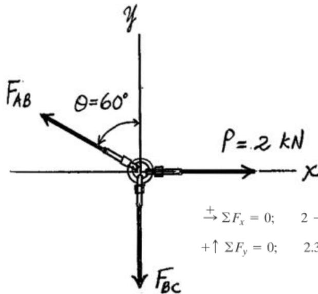
$$\rightarrow \Sigma F_x = 0; \quad 2 - F_{AB} \sin 60^\circ = 0 \quad F_{AB} = 2.309 \text{ kN}$$
