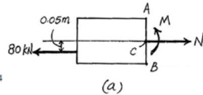
The normal stress developed is the combination of axial and bending stress
