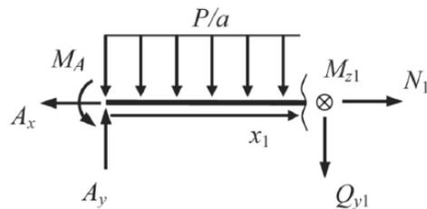
$$\begin{aligned} \sum F_x : \quad & \underline{N_1(x_1) = A_x = P} \\ \sum F_y : \quad & \underline{Q_{y1}(x_1) = A_y - \frac{P}{a}x_1 = \frac{3P}{2} - \frac{P}{a}x_1} \\ \sum M_{z1} : \quad & M_{z1} - M_A + A_y x_1 - \frac{P}{a}x_1 \frac{x_1}{2} = 0 \end{aligned}$$
