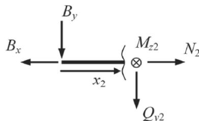
$$\begin{aligned} \sum F_x : \quad & \underline{N_2(x_2) = B_x = P} \\ \sum F_y : \quad & \underline{Q_{y2}(x_2) = -B_y = -\frac{P}{2}} \\ \sum M_{z1} : \quad & M_{z2} - B_y x_2 = 0 \end{aligned}$$
