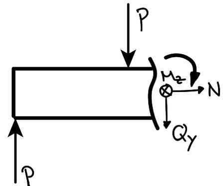
$$\sigma_{top,max} = -\frac{M_{z,max} \cdot (\Delta y_{top,max})}{I_z} = -\frac{(-1.5 \cdot 10^3)(-0.035)}{512.5 \cdot 10^{-9}} = -102.4 \text{MPa} \Rightarrow \sigma_{max,druck}$$
