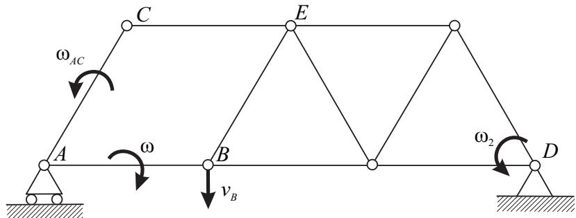
$$v_B = l \omega = 2l \omega_2 \quad \Rightarrow \quad \omega_2 = \frac{\omega}{2}$$
