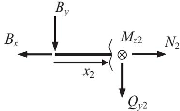
$$\begin{aligned} \sum F_x : \quad N_2(x_2) &= B_x = P \\ \sum F_y : \quad Q_2(x_2) &= -B_y = -\frac{1}{2}P \\ \sum M_z : \quad M_{z2}(x_2) &= B_y x_2 = \frac{1}{2}P x_2 \end{aligned}$$
