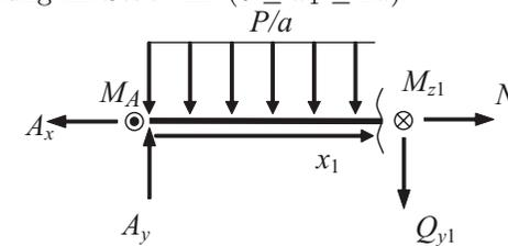
$$\begin{aligned} \sum F_x: \quad & N_1(x_1) = A_x = P \\ \sum F_y: \quad & Q_1(x_1) = A_y - \frac{P}{a}x_1 = \frac{3}{2}P - \frac{P}{a}x_1 \\ \sum M_z: \quad & M_{z1}(x_1) = M_A - A_yx_1 + \frac{P}{a}x_1 \frac{x_1}{2} = aP - \frac{3}{2}Px_1 + \frac{P}{2a}x_1^2 \end{aligned}$$
