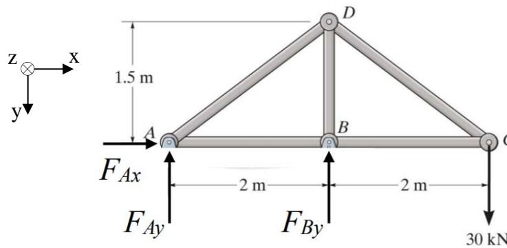
$$\sum F_x = 0 \rightarrow F_{Ax} = 0, \quad \sum M_B = 0 \rightarrow F_{Ay} = -30\text{kN}, \quad \sum F_y = 0 \rightarrow F_{By} = 60\text{kN}$$
