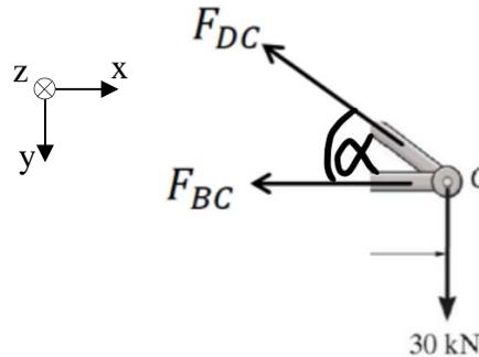
$$\sum F_y = 0 \rightarrow F_{DC} = \frac{30\text{kN}}{\sin \alpha} = 50\text{kN}, \quad \sum F_x = 0 \rightarrow F_{BC} = -\cos \alpha F_{DC} = -40\text{kN}$$
