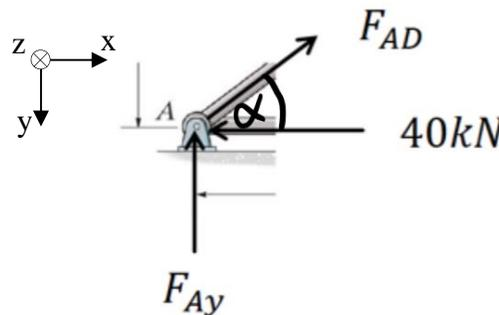
$$\sum F_x = 0 \rightarrow F_{AD} = \frac{40\text{kN}}{\cos \alpha} = 50\text{kN}$$
