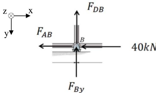
$$\sum F_x = 0 \rightarrow F_{AB} = -40\text{kN}, \quad \sum F_y = 0 \rightarrow F_{DB} = -F_{By} = -60\text{kN}$$
