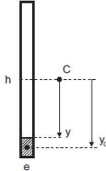
$$H_z^{Steg}(y) = H_z(\bar{z}) + y_c(y) \cdot dA(y) = \frac{eah}{2} + \frac{1}{2} \left( \frac{h}{2} + y \right) \left( \frac{h}{2} - y \right) e = \left( ah + \frac{h^2}{4} - y^2 \right) \frac{e}{2}$$
