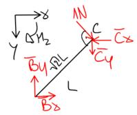
$$\sum F_x = 0 \to \overline{C}_x = \frac{\sqrt{2}}{2}N + \overline{B}_x, \\ \sum F_y = 0 \to \overline{C}_y = \overline{B}_y - \frac{\sqrt{2}}{2}N, \\ \sum M_C = 0 \to \overline{B}_x = \overline{B}_y$$
