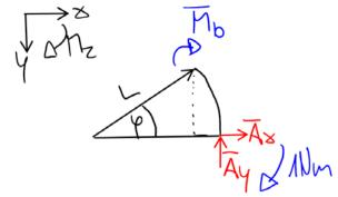
$$\sum M = 0 \to \overline{M}_b(\varphi) = \frac{1Nm}{2} (\sin \varphi - \cos \varphi - 1)$$
