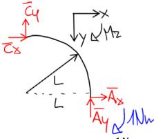
$$\sum M_A = 0 \to \overline{B}_x = -\frac{1Nm}{2L}, \qquad \sum F_x = 0 \to \overline{A}_x = \frac{1Nm}{2L}, \qquad \sum F_y = 0 \to \overline{A}_y = \frac{1Nm}{2L}$$
