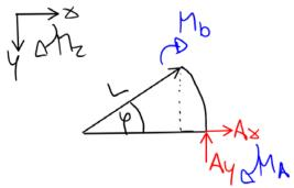
$$\sum M = 0 \to M_b(\varphi) = L \left[ B_x - \left( \frac{P}{2} - B_x \right) \cos \varphi - B_x \sin \varphi \right]$$
