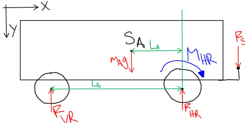
$$\begin{aligned}\sum F_y = 0 &\rightarrow F_{VR} = m_A g + F_S - F_{HR}, \\ \sum M_{z,VR} = 0 &\rightarrow F_{HR} = \frac{m_A g(L_5 - L_4) + M_{HR} + F_S(L_5 + L_3)}{L_5} \\ &\rightarrow F_{VR} = \frac{-M_{HR} - L_3 F_S + L_4 m_A g}{L_5}\end{aligned}$$
