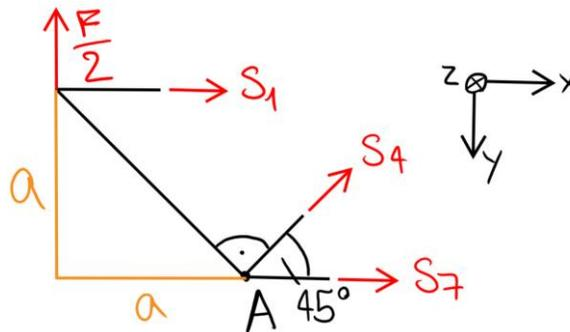
$$\begin{aligned} \sum M_A = 0 &\rightarrow S_1 = -32\text{kN} = S_2, & \sum F_y = 0 &\rightarrow S_4 = -45.255\text{kN} = S_3 = S_5 = S_6, \\ \sum F_x = 0 &\rightarrow S_7 = -64\text{kN} \end{aligned}$$
