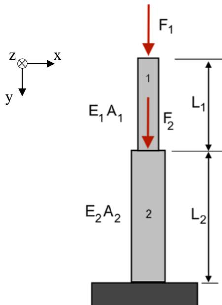
Gegeben:  $F_1 = 12\text{kN}$ ,  $F_2 = 9\text{kN}$ ,  $A_1 = 80\text{cm}^2$ ,  $L_1 = 30\text{cm}$ ,  $L_2 = 40\text{cm}$ ,  $E_2 = 210\text{GPa}$
