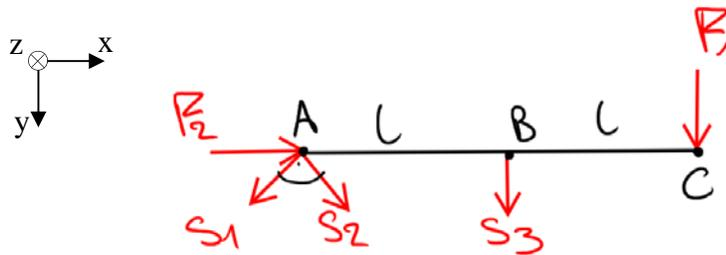
$$\begin{aligned} \sum M_A = 0 &\rightarrow S_3 = -2F_1, \\ \sum F_x = 0 \text{ \& } \sum F_y = 0 &\rightarrow S_1 = \frac{\sqrt{2}}{2}(F_2 + F_1), \quad S_2 = \frac{\sqrt{2}}{2}(F_1 - F_2) \end{aligned}$$
