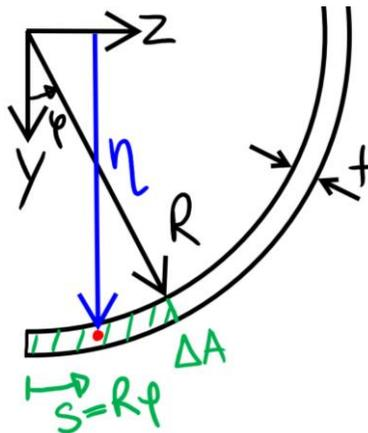
$$H_z(\varphi) = \eta \cdot \Delta A \approx R \cos\left(\frac{\varphi}{2}\right) \cdot R t \varphi = R^2 t \varphi \cos\left(\frac{\varphi}{2}\right)$$
