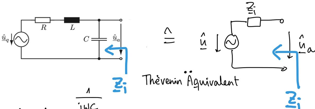
$$\underline{\hat{u}} = \underline{\hat{u}}_a = \underline{\hat{u}}_g \cdot \frac{\frac{1}{j\omega C}}{\frac{1}{j\omega C} + R + j\omega L} = (60.98 - j48.9) \text{ V}$$
