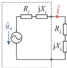
$$\underline{S} = \frac{1}{2} \hat{u} \hat{i}^* = P + jQ = U \cdot I e^{j\Delta\varphi} = S e^{j\Delta\varphi} = \sqrt{P^2 + Q^2} e^{j\Delta\varphi}$$
