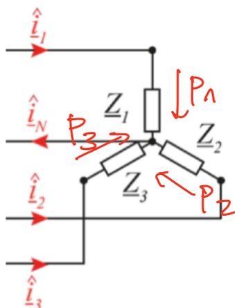
$$\underline{\hat{i}}_1 = \frac{\underline{\hat{u}}_1}{\underline{Z}_1} = \frac{\underline{\hat{u}}_1}{R_1 + j\omega L_1}$$
