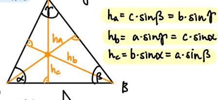
$$\begin{aligned} h_a &= c \cdot \sin \beta = b \cdot \sin \gamma \\ h_b &= a \cdot \sin \gamma = c \cdot \sin \alpha \\ h_c &= b \cdot \sin \alpha = a \cdot \sin \beta \end{aligned}$$
