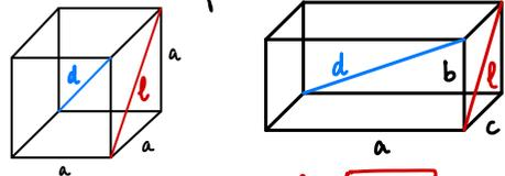
$$\begin{aligned} \text{Quader: } l &= \sqrt{2}a, d = \sqrt{3}a \\ \text{Würfel: } l &= \sqrt{b^2 + c^2}, d = \sqrt{a^2 + b^2 + c^2} \end{aligned}$$
