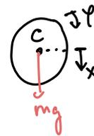
$$\begin{aligned} m\ddot{x} &= mg \\ \dot{L}_c &= I_0 \dot{\psi} = 0 \end{aligned}$$
