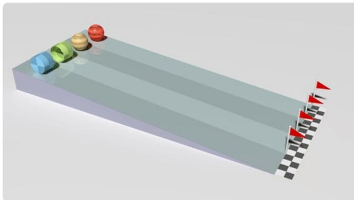
Four objects with identical masses and radii racing down a plane while rolling without slipping. □
