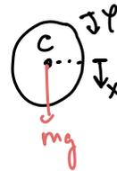
$$\begin{aligned} m\ddot{x} &= mg \\ \dot{L}_c &= I_0\ddot{\psi} = 0 \end{aligned}$$
