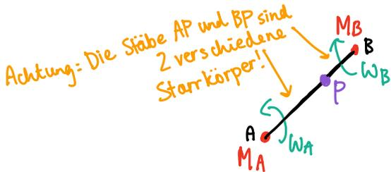
$$\frac{\omega_A}{\omega_B} = \frac{r_{BP}}{r_{AP}}$$
