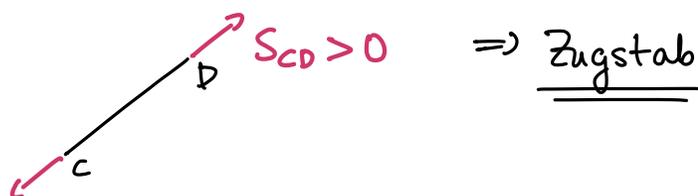
$\textcircled{4} \Rightarrow S_{BD} = -\frac{\sqrt{2}}{2} S_{AD} - \frac{\sqrt{2}}{2} S_{CD} \quad / \quad S_{AD} = S_{CD} = \frac{\sqrt{2}}{2} F$
