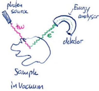
ARPES is a technique which uses the photoelectric effect and can be used to determine the hole dispersion relation. A photon is fired at the sample where its energy is transferred to the ejected electron and the quasi hole left behind. One can then plot the quasi hole energy vs the quasi hole momentum to get the dispersion relation.
