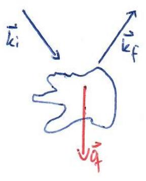
Diffraction is the tool of choice to study phase transitions where the order parameter is a particular spatial Fourier component of some microscopic density.  $\Rightarrow I_q \sim |g_q|^2$
