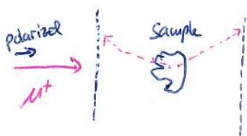
Muon spin spectroscopy is an experimental technique based on the implantation of spin-polarized muons in matter and on the detection of the influence of the atomic or crystalline surroundings on their spin motion. The motion of the muon spin is due to the magnetic field experienced by the particle and may provide information on its local environment.
