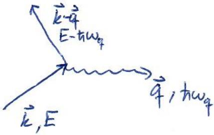
Neutron spectroscopy is a powerful technique to study phonon dispersion curves. A high count rate means that at that particular momentum  $\vec{q}$  it is possible to excite a phonon with that particular energy  $\hbar\omega$ .
