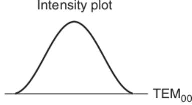
Figure 16: Intensity in the transverse direction of a Gaussian beam. [11]
