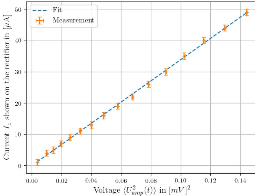
Figure 7: Scatter plot of the measured values shown in Table 6, whereupon the Voltage  $\langle U_{amp}^2(t) \rangle$  was squared before plotting. The gradient of the linear regression is the quantity  $G_I$ . The error bars of the Voltage  $\langle U_{amp}^2(t) \rangle$  are not clearly visible as they are smaller than the marker.
