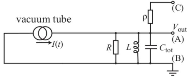
Figure 3: Schematic of the LC-circuit at resonance frequency. The second connection (C) which was not shown in Figure 1 is not used for the final measurement but for initial measurements such as the measurement of the resonance frequency, the total capacitance and the resistance. Image from [1].
