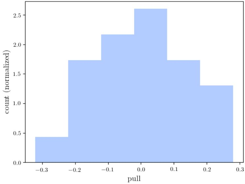
Figure 6: The theory proposes a linear dependency of the resistance  $R$  on the diode current  $\langle I \rangle$ . Using the method of least squares a first order polynomial curve was fitted in the data (See Figure 5). This histogram shows the deviation of the fitted curve from the measured values. The numbers of bins  $k$  was calculated using Equation (13) and was set to 6. The histogram was normalized to the area of 1.
