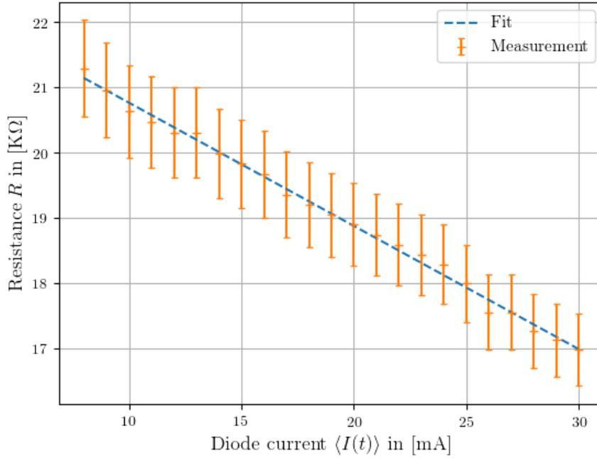
Figure 5: Scatter plot for the determination of the resistance  $R$  with the acquired data in Table 5.
