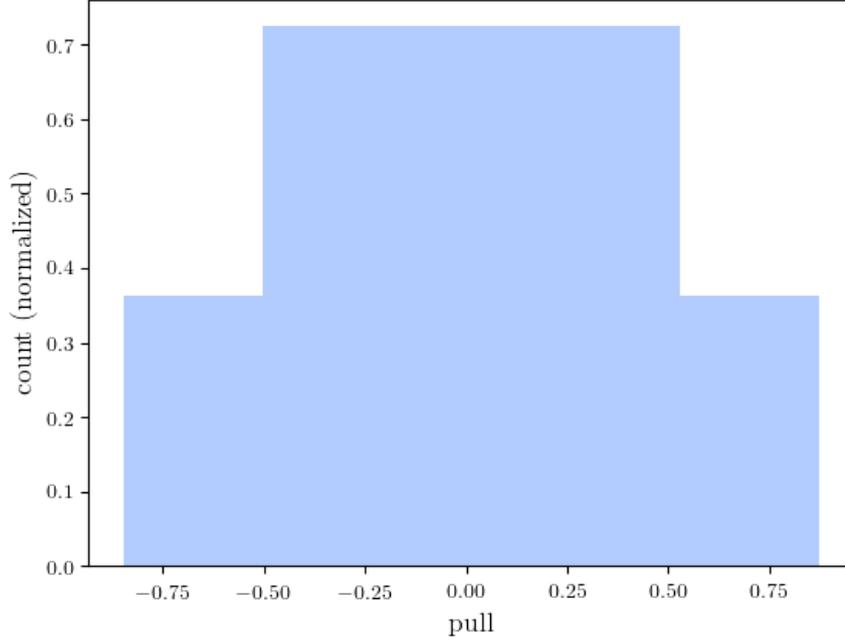
Figure 8: The theory proposes a linear dependency of the current  $I_z$  on the voltage  $\langle U_{amp}^2(t) \rangle$ . Using the method of least squares a first order polynomial curve was fitted in the data (See Figure 7). This histogram shows the deviation of the fitted curve from the measured values. The numbers of bins  $k$  was calculated using Equation (13) and was set to 5. The histogram was normalized to the area of 1.
