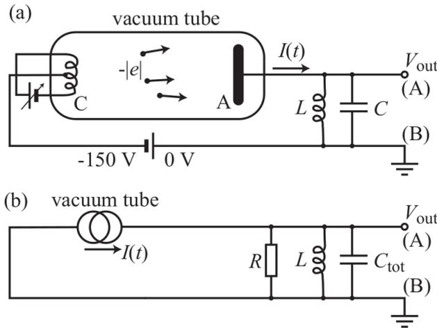
Figure 1: In (a) the schematic of the noise generator which is used to generate and filter shot noise at a specific frequency. In (b) the resistance of the LC-circuit is drawn as an ohmic resistance, whereat this only holds for signals at resonance frequency.
