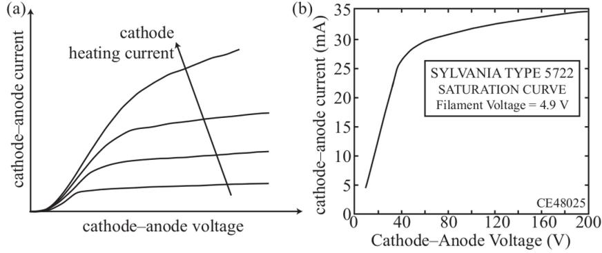
Figure 2: The cathode heating current is a dc-current and is shown in Figure 1 (a) at the cathode (C). In this experiment, the voltage applied on the diode is 150V which is in the saturation region of the diode, i.e., the cathode-anode current has negligible dependence on the cathode-anode voltage. Illustration from [1].
