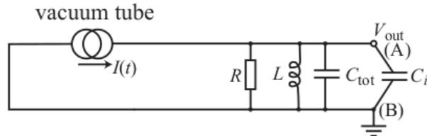
Figure 4: Schematic of the LC-circuit in order to measure the total capacitance  $C_{tot}$ . The second capacitance  $C_i$  is connected into (A). Image from [1].
