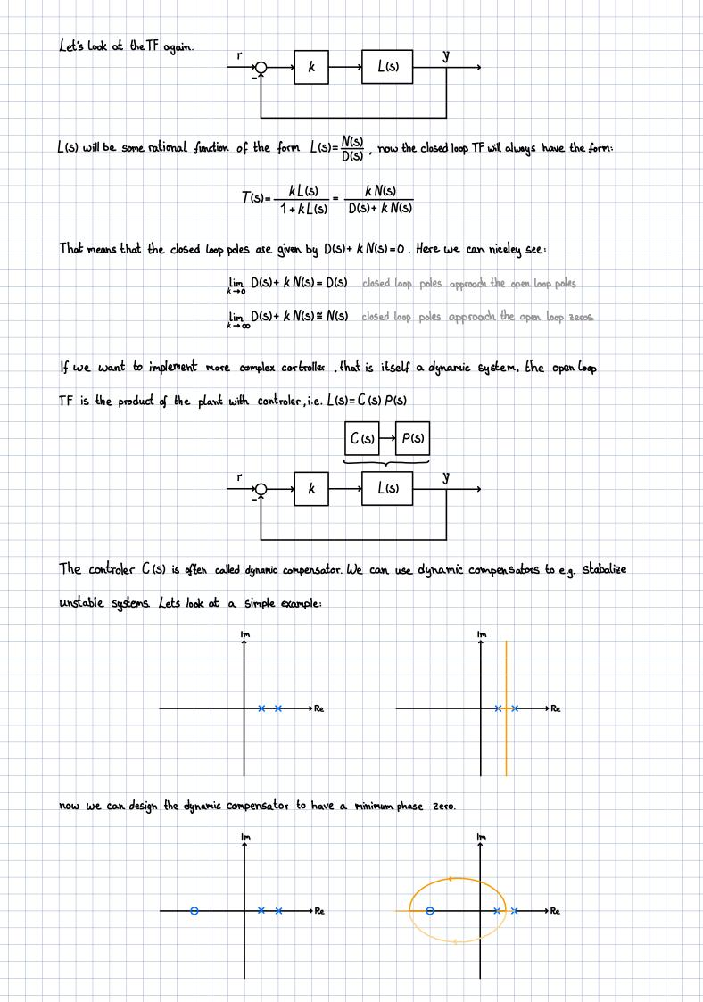
By adding a zero we are able to make the feedback connection stable. This is also called a PD controler.
