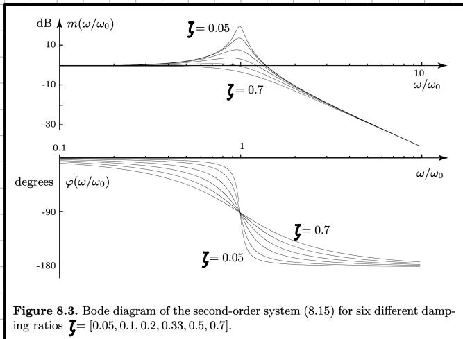
Figure 8.3. Bode diagram of the second-order system (8.15) for six different damping ratios  $\zeta = [0.05, 0.1, 0.2, 0.33, 0.5, 0.7]$ .
