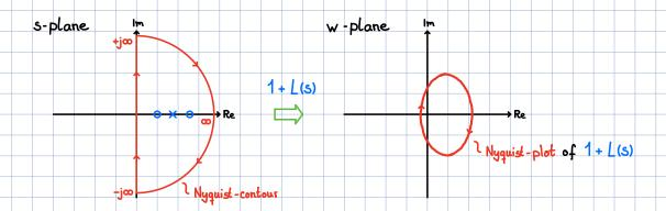
By choosing our contour like this we can tell the relative difference of poles and zeros of 1 + L(s) in the RHP by counting the encirclements of the Nyquist-plot of 1 + L(s), arround the origin. A nice characteristic of the Nyquist-plot is that:
