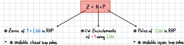
We can now asses wether a closed loop system is stable, by only looking at the OL poles and the Nyquist-plot
