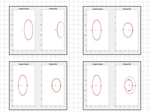
What we can see is that for every time we encircle a pole/zero in the s-plane we also encircle the origin in the w-plane. For each clockwise encirclement of zeros we get one CW encirclement of the origin, and for each CW encirclement of a pole we get one CCW encirclement of the origin.
