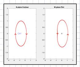
This means that you can tell the relative difference of poles and zeros inside a contour by how many times the plot circles the origin and in which direction.
