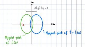
So instead of counting the encirclements of 1+ L(s) arround zero, we can shift the coordinate system by -1 and count the encirclements of L(s) arround -1. This is nice since we know how to draw the Nyquist-plot of L(s).
