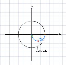
To draw these plots it is usefull to look at special points e.g.  $\omega + 0$  and  $\omega + \infty$ , also the intersection(s) with the unit circle and imaginary and real axes. Today we will expand and go further with the polar plot.
