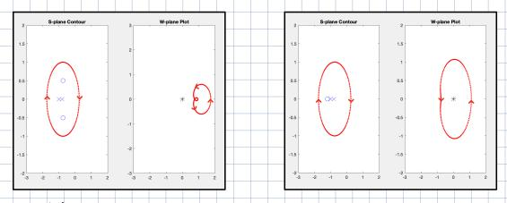
This means that you can tell the relative difference of poles and zeros inside a contour by how many times
