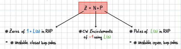
We can now asses wether a closed loop system is stable, by only looking at the OL poles and the Nyquist-plot
