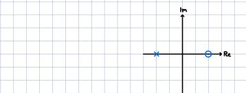
This means for large enough gains the closed loop will become unstable. A n.m.p. zero also limits the maximum crossover freq. The consequence is that the CL system becomes slow.
