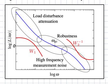
Next to high-and low-frequency behavior we can also constrain the bandwidth of CL system. The bandwidth tells us the maximum frequency for which the output can track commands within a factor  $\approx 0.7$ . In other words the bandwidth tells us for which max freq. we get satisfactory operation. ( $|T(j\omega)| > \sqrt[1]{2}$ )
