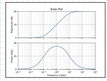
Example for a = 0.1, b = 10, i.e.  $C_{lead}(s) = \frac{10s+1}{0.1s+1} = 100 \frac{s+0.1}{s+10}$
