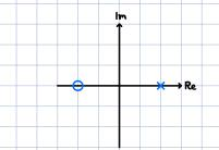
We need a high gain to stabolize the system In real life a high gain means fast and strong actuators.
