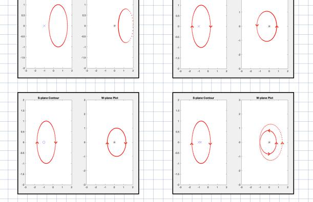
What we can see is that for every time we encircle a pole/zero in the s-plane we also encircle the origin in the w-plane. For each clockwise encirclement of zeros we get one CW encirclement of the origin, and for each CW encirclement of a pole we get one CCW encirclement of the origin.
