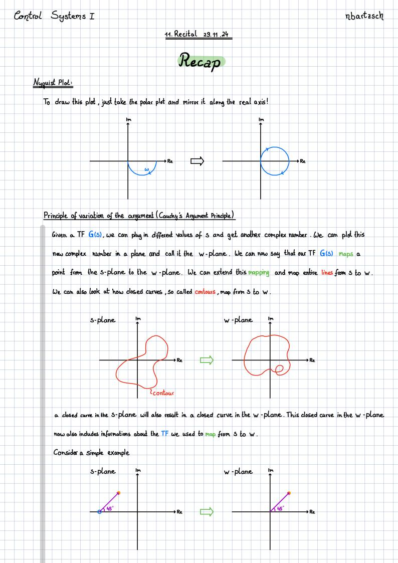
We observe that the phasor of the point in the w-plane is the same as the one from the zero to the original point in the S-plane. Let's add in a pole and see what happens:
