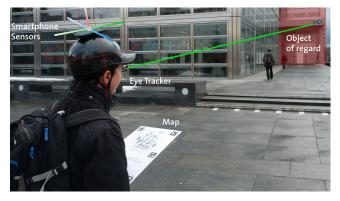
Figure 1. Object of regard identification through eye, location and head tracking.
